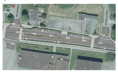
Remodeling Peninsula Road will allow for designated parking spaces, and a wider road width. Concept plans have been developed by McElhanney and presented to the District. This will include additional sidewalks, bike lanes and increased driving lanes. This design will not provide any additional safety measures but will
